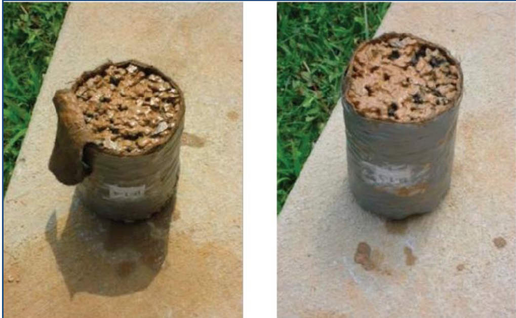
Figure 4-6. Specimen After Exposure to Clayey Silty Sand (Adapt from [28])
