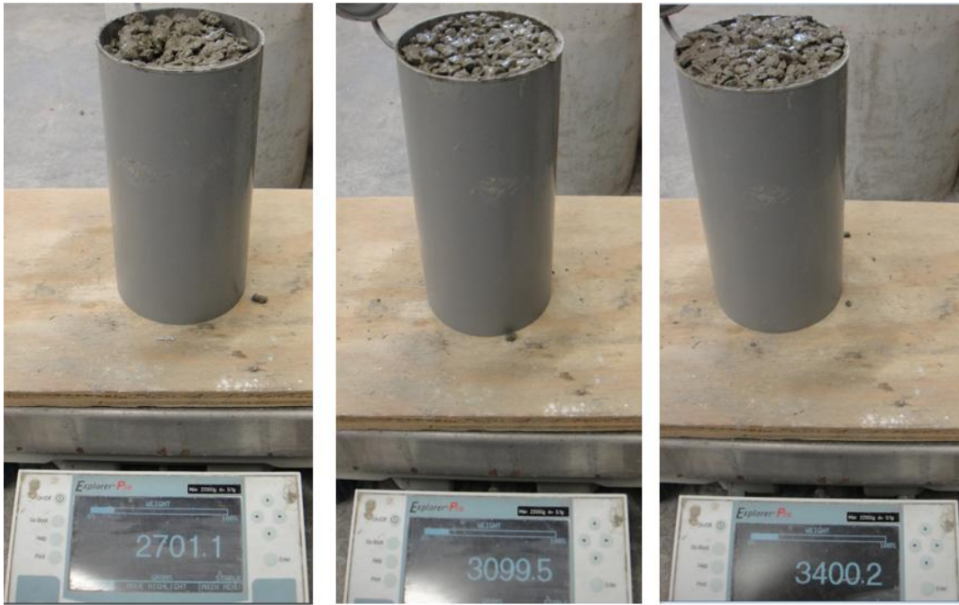
Figure 3-3. Different Amount of Fresh Filling Material in Each Mold Compacted by Roding and Tapping Method to Achieve Designed Porosity
