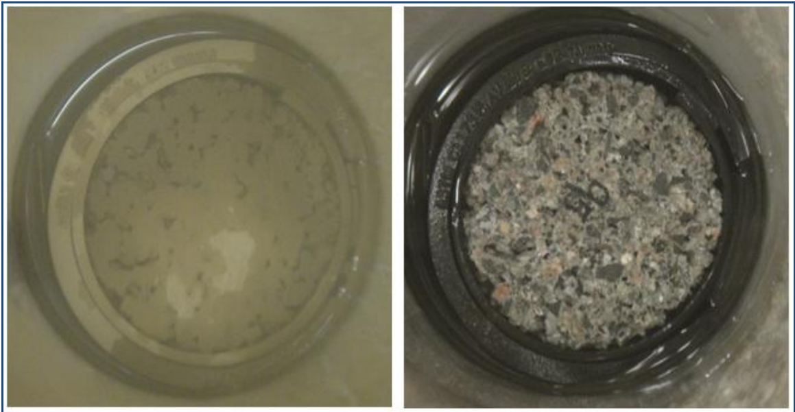
Figure 4-2 Specimens at Exposure to Clayey Silt in This Study (Left: Before Test; Right: After Test)
