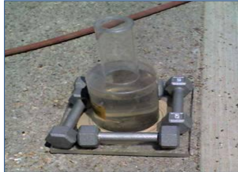
Figure 2-12. Field Permeameter Setup
