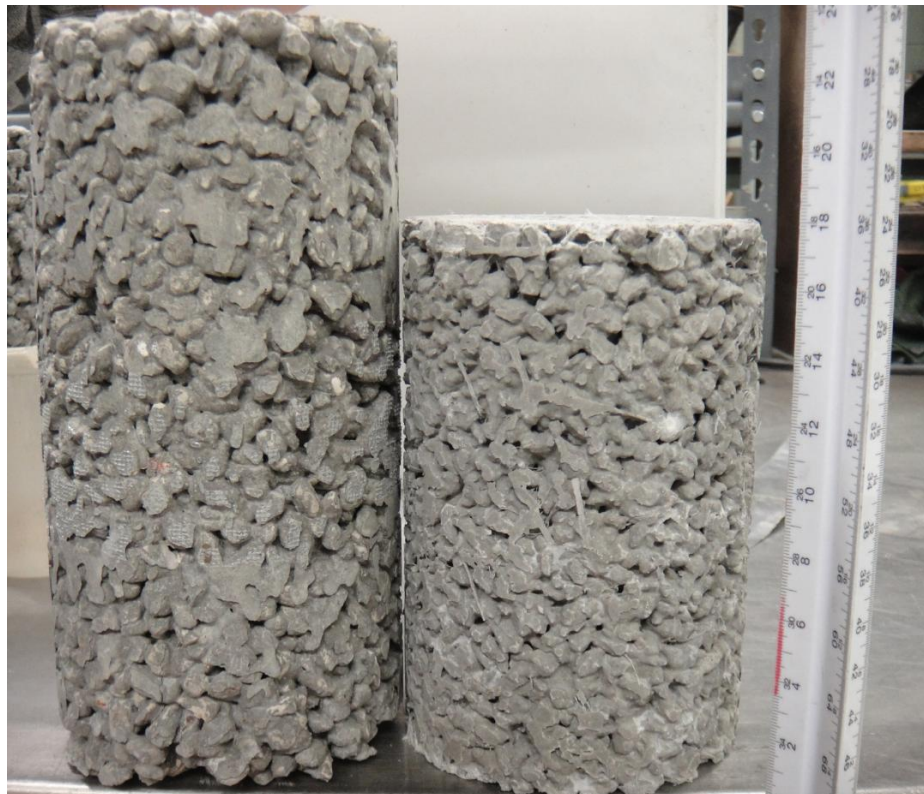
Figure 3-2. Untrimmed Specimen (Left) and Trimmed Specimen (Right)
