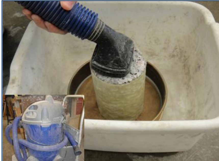
Figure 3-7. Vacuuming the Clogged Specimen
