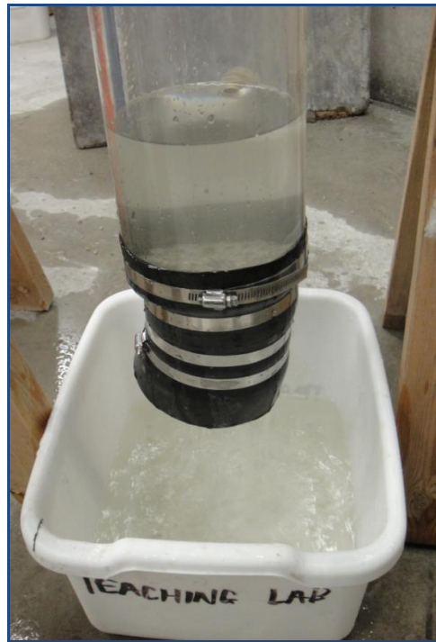
Figure 4-11. Sand Sedimentation Test is in Progress
