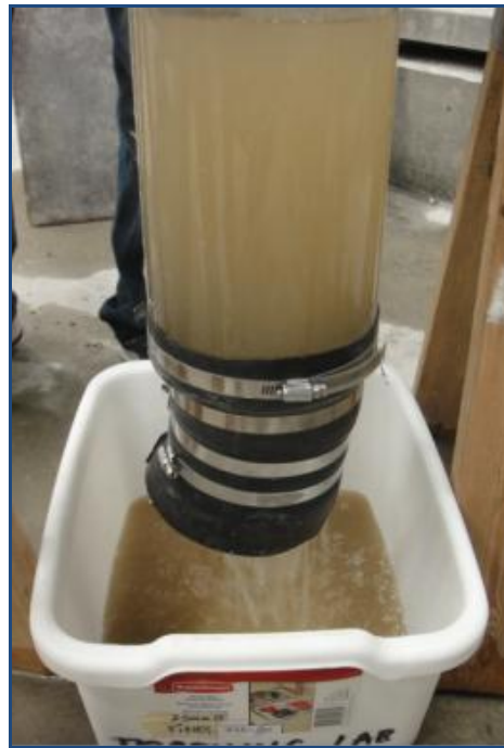
Figure 4-15. Clay Silty Sand Sediments Is In Progress
