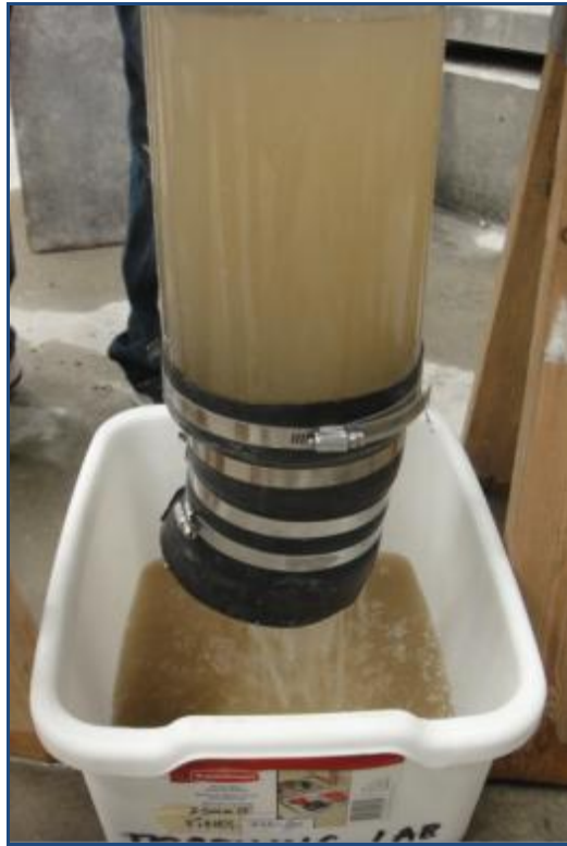
Figure 4-3. The Clayey Silt Sedimentation Test is in Progress
