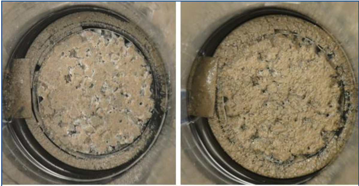
Figure 4-14. Specimens Exposed to Clayey Silty Sand Sediments before (Left) and after Sedimentation Test
