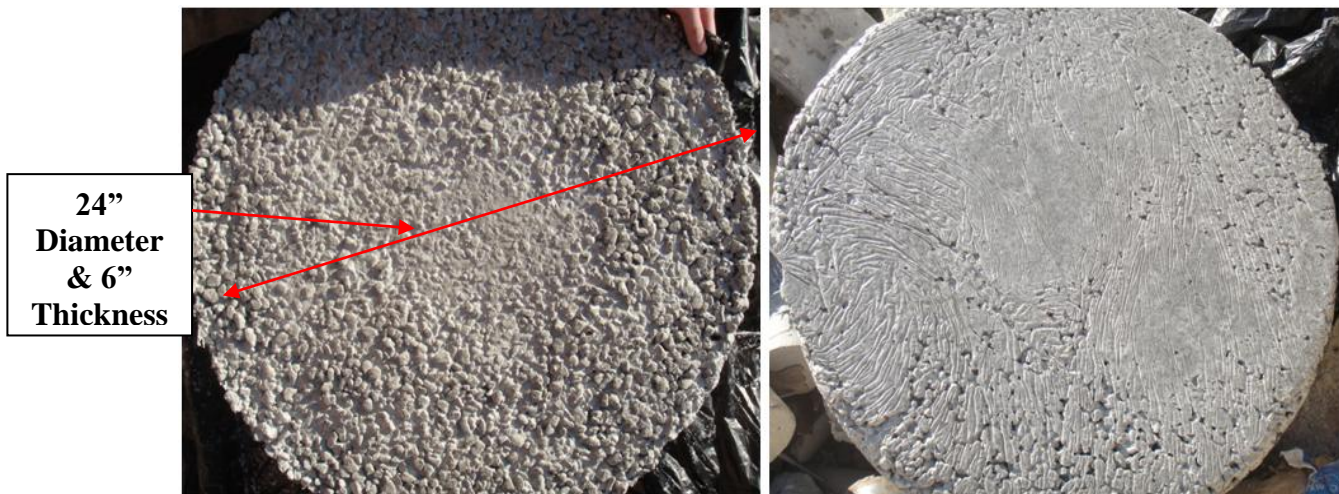
Figure 2-3. Excessive Water Leading to Segregation of PCPC Slab: Top View (Left) & Bottom View (Right)
