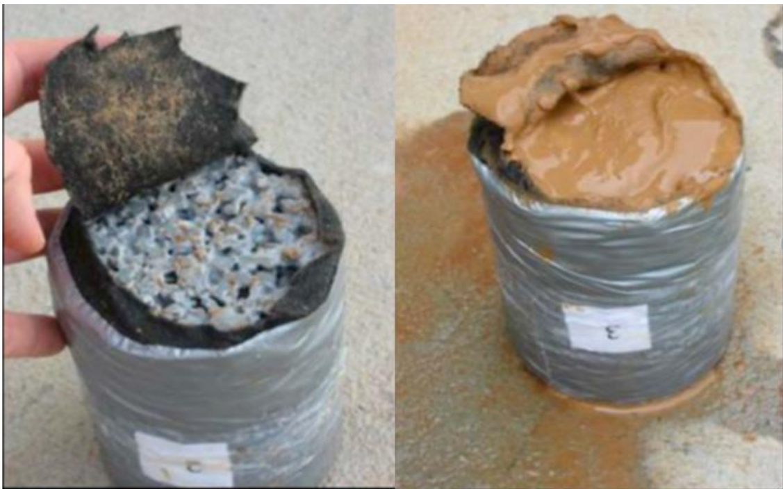
Figure 2-26. Pervious Concrete Specimens Subjected to Sand (Left) and Clay (Right) as Sedimentation Materials (Adopted from [28])
